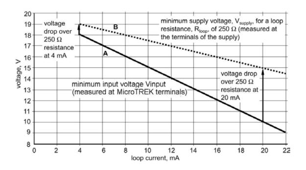
Line A = minimum voltage at the GWR-1000 2-wire terminals Line B = minimum supply voltage (for voltage drop caused by a 250 Ohm loop resistance)
