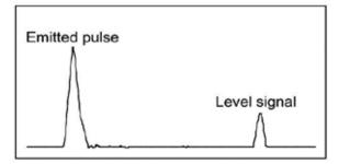
Coaxial probe with gain 1
