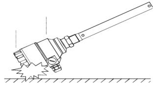
Avoid bending (single rod and coaxial probes) -Support the probe to avoid bending.
