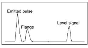
Rod or cable probe with gain 2
