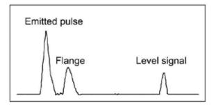
Rod or cable probe with gain 1
