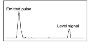
Coaxial probe with gain 2
